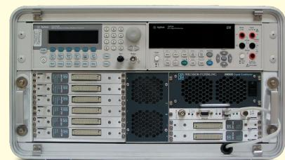
**Qty. 4 28000-TEST Test Subsystem for performing system validation and in-situ NIST traceable calibrations**
